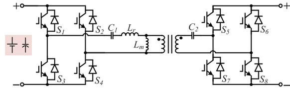
Fig. 19. CLLC DC/DC converter.
