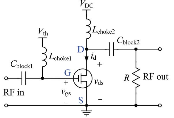
Fig. 5. Circuit of class B power amplifier.
