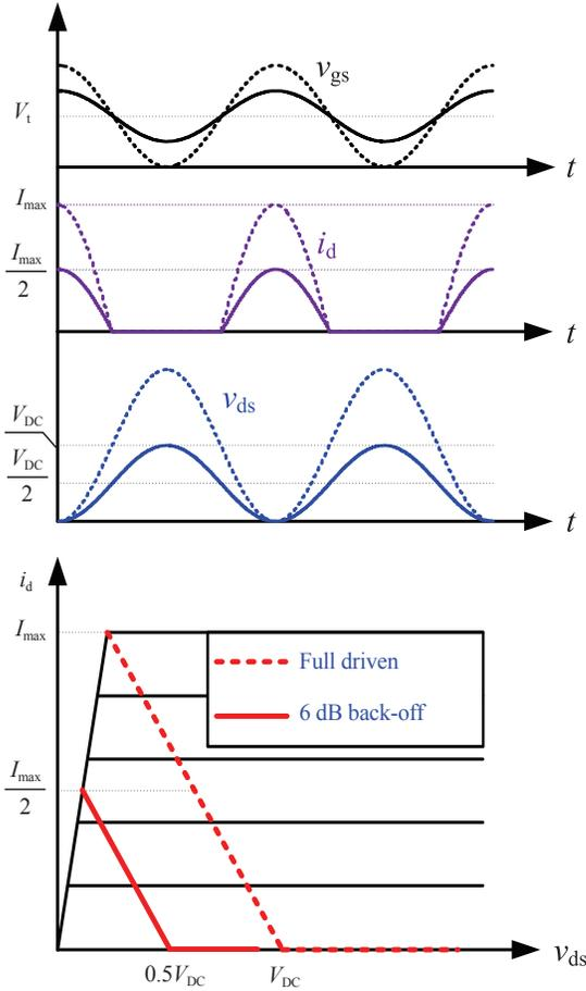
Fig. 10. Voltage and current waveforms and load lines of class B power amplifiers using ET technique at different power levels.
