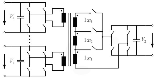
Fig. 11. Dual-active bridge converter with tap changer.
