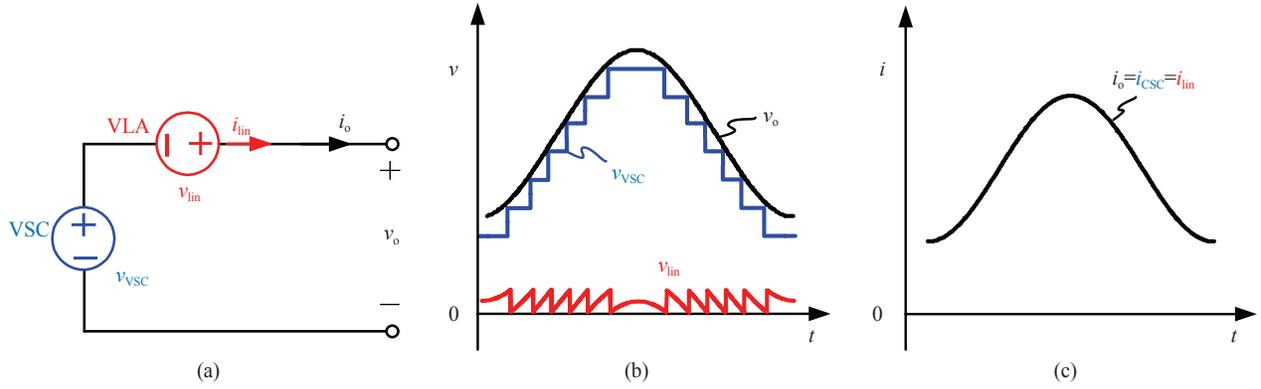
Fig. 18. Block diagram and key waveforms of series-form SLH ET power supply. (a) Block diagram. (b) Key voltage waveforms. (c) Key current waveforms.
