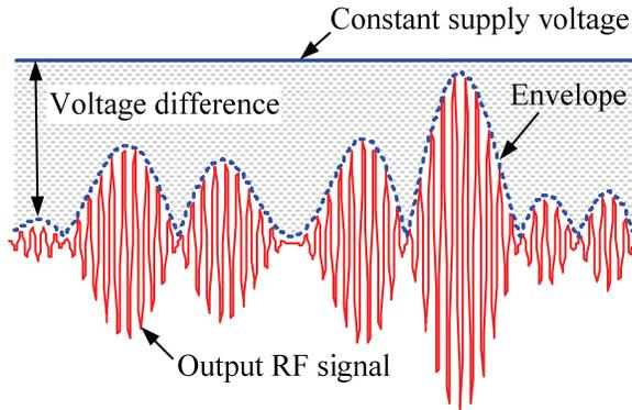
Fig. 2. Key waveforms of the LPA in 3G and 4G mobile communication systems.
