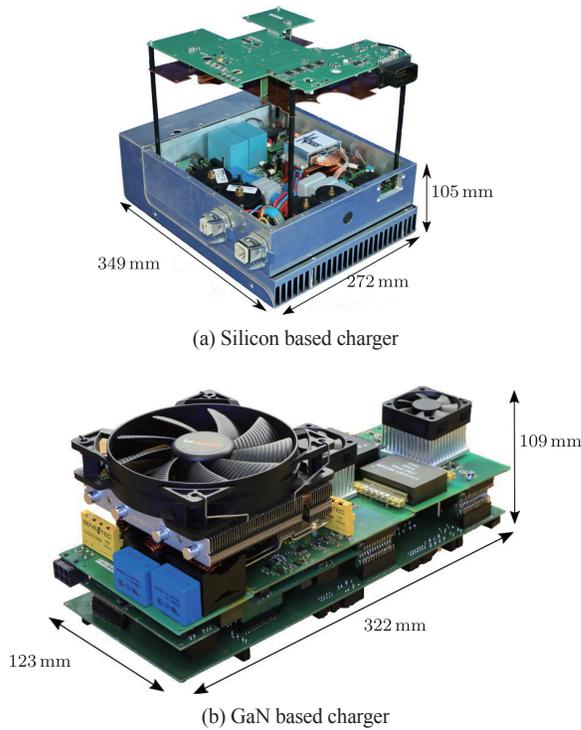
Fig. 15. Comparison of a Silicon and a GaN based battery charger.
