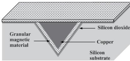
Fig. 23. Schematic of a V-groove inductor [110].
