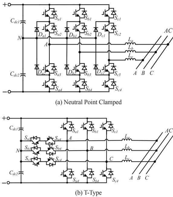
Fig. 21. Neutral point clamped multilevel DC-AC converter.
