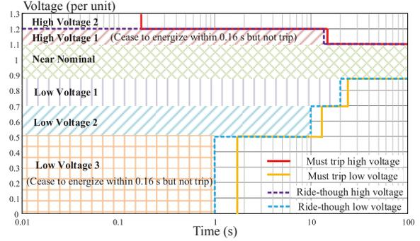
Fig. 10. Voltage ride-through requirements.
