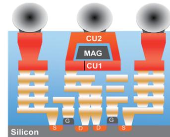
Fig. 10. Illustrated cross section of magnetic thin-film inductors integrated with CMOS IC.
