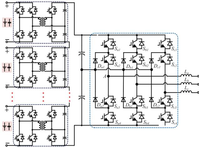
Fig. 25. Series DC bus configuration.
