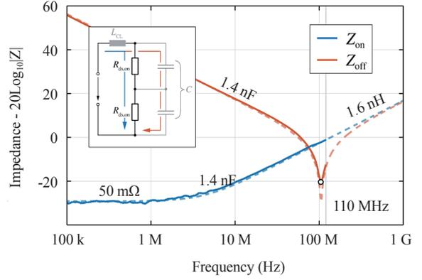
Fig. 2. Impedance measured from the DC terminals of the PM shown in Fig. 1 when (blue) both MOSFETs are conducting and (red) blocking. Series  $RL$  and  $LC$  equivalent circuits (dashed) with the values given in the figure match the measurements respectively. For frequency higher than 110 MHz, only the simulated curves converging to  $L_{CL} = 1.6$  nH are shown.
