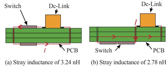
Fig. 17. Stray inductances as a result of different layouts.
