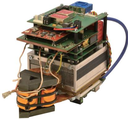
Fig. 9. Photograph of an air-cooled, galvanically isolated three-phase dual-active bridge dc-dc converter. Volume with housing around 2.4l.
