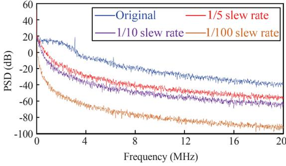
Fig. 24. Power spectral density of envelope signals with different slew rate.
