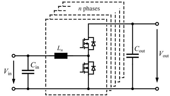
Fig. 2. Multi-phase boost converter.
