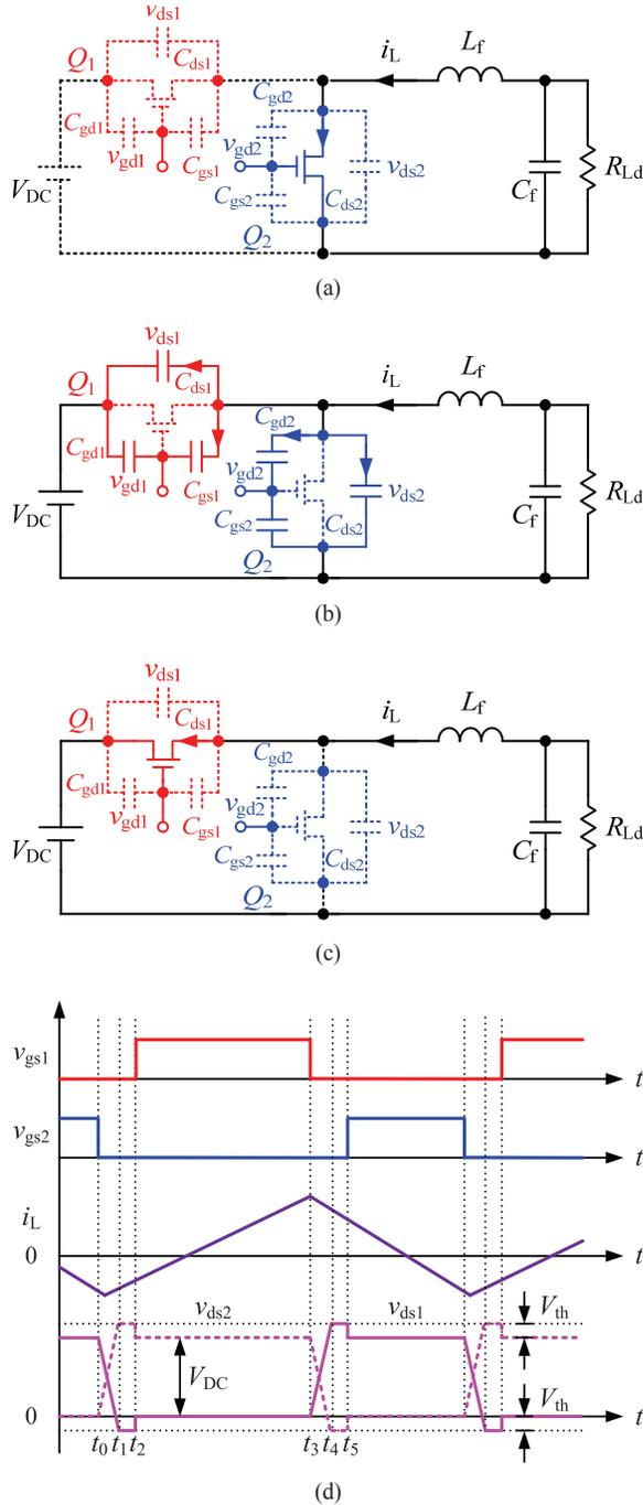
Fig. 22. Equivalent circuits and key waveforms of the buck converter. (a) Equivalent circuit before  $t_0$ . (b) Equivalent circuit during  $[t_0, t_1]$ . (c) Equivalent circuit during  $[t_1, t_2]$ . (d) Key waveforms.
