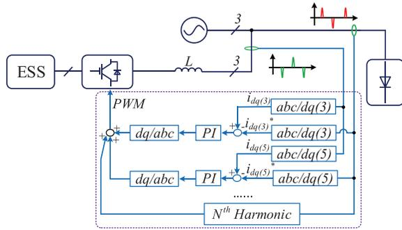
Fig. 12. Harmonics compensation control diagram.
