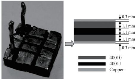
Fig. 28. Prototype of the nonlinear LTCC inductor [125].
