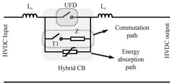
Fig. 5 Hybrid HVDC circuit breaker ( $L_s$ - refers to network inductance).
