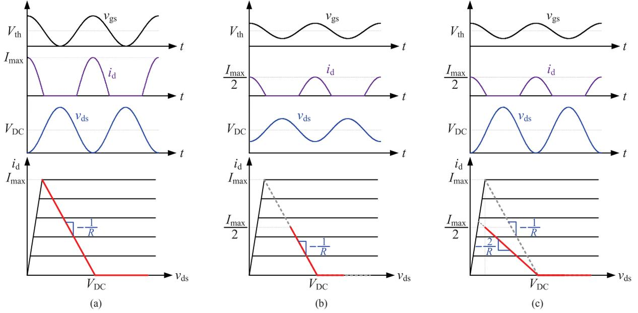
Fig. 6. Voltage and current waveforms and load lines of class B power amplifiers. (a) Full driven with load resistance  $R$ . (b) 6 dB back-off with load resistance  $R$ . (c) 6 dB back-off with load resistance  $2R$ .
