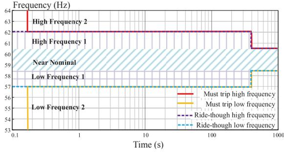
Fig. 11. Frequency-ride through requirements.
