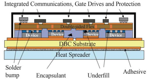
Fig. 3. Flip-Chip based module structure [20].
