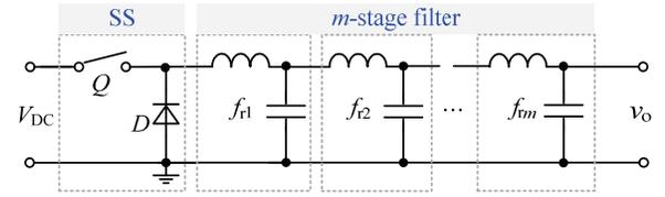
Fig. 14. Buck converter with  $m$ -stage filters.
