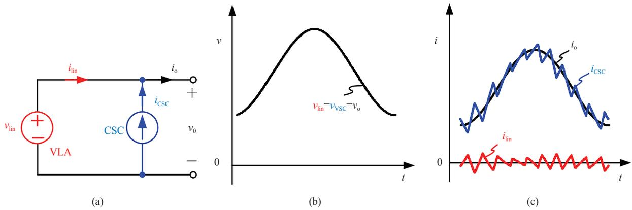
Fig. 19. Block diagram and key waveforms of parallel-form SLH ET power supply. (a) Block diagram. (b) Key voltage waveforms. (c) Key current waveforms.
