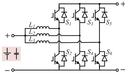
Fig. 17. Bidirectional interleaved DC-DC converter.
