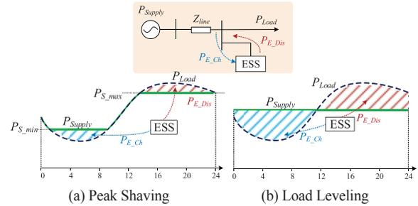
Fig. 6. Peak shaving &amp; load leveling function.
