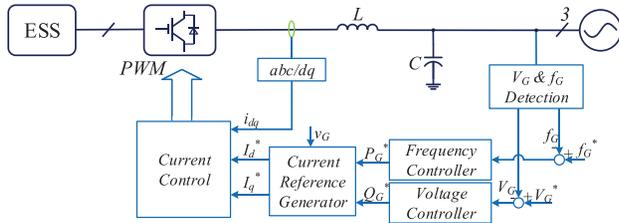
Fig. 9. Voltage & frequency regulation control diagram.
