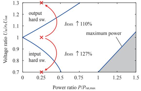
Fig. 8. Exemplary soft-switching boundaries and changes of RMS current of a single-phase DAB converter.
