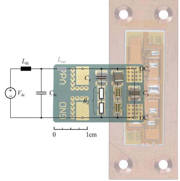
Fig. 3. 1 mm-thick PCB providing a practical and low inductive solution to integrate the buffer capacitor  $C_b$  and the damping network  $R_d C_d$  in the PM. One undamped and two damped 1210 *Kemet<sup>TM</sup>* 1500 V *X7R* ceramic capacitors find place together with power resistors of different values.
