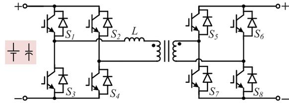
Fig. 18. Bidirectional dual active bridge DC-DC converter.
