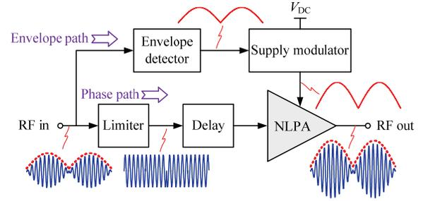
Fig. 8. Schematic diagram and key waveforms of EER technique.
