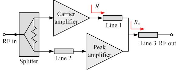
Fig. 4. Schematic diagram of the even Doherty amplifier.
