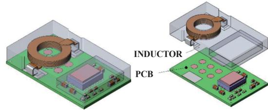
Fig. 26. Schematic of a power-system-in-inductor module [113].
