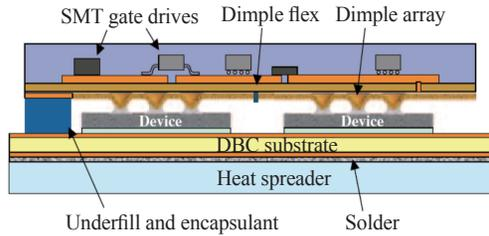
Fig. 4. DAI based module structure [20].
