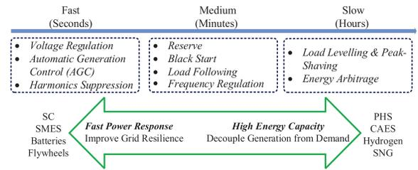
Fig. 5. Grid support function diagram.
