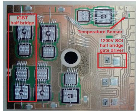
Fig. 12. A 1200 V/50 A module with integrated gate drive and temperature sensor [55].
