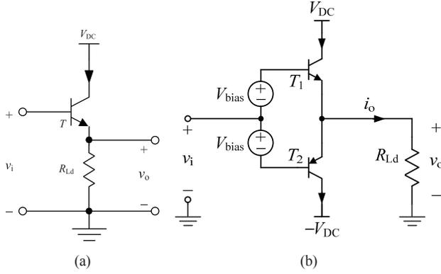
Fig. 12. Circuits of typical linear amplifiers. (a) Class A. (b) Class AB.
