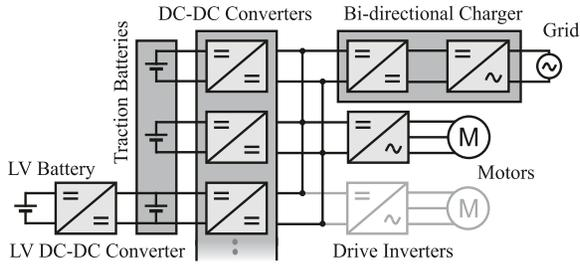
Fig. 1. Modular propulsion system architecture.
