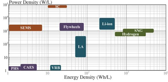
Fig. 3. Power and energy density comparison for ESSs.
