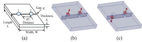
Fig. 15. Two-phase lateral-coupled inductor structure [74]. (a) Dimensions. (b) Direct coupling. (c) Inverse coupling.
