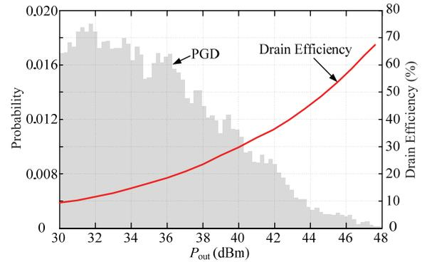
Fig. 3. DE curve of the LPA when powered by 28 V constant voltage and PGD of the RF output signal versus the output power.
